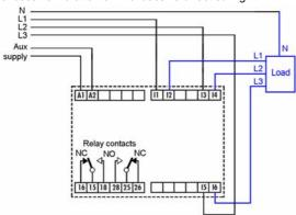
NC = Normally closed. Contact closed when relay de-energised.NO = Normally open. Contact open when relay de-energised.
