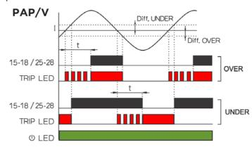
The time delay and differential trip levels help to prevent relay chatter as the monitored current level varies. As the relays have changeover contacts, the relay outputs can be inverted by wiring to the alternative terminals 15-16 or 25-26.
